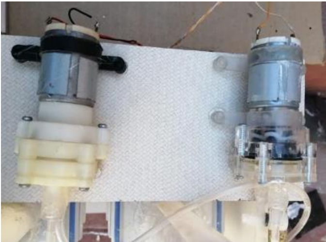
Figure 7: 12V diaphragm pump for gas collection. To demonstrate that hydrogen gas is pure, the gas produced was extracted through a controlled nozzle, which is seen in Figure 8. In this experiment, the gas flame remains constant and does not produce an explosion, since it only encounters oxygen when leaving the nozzle.
